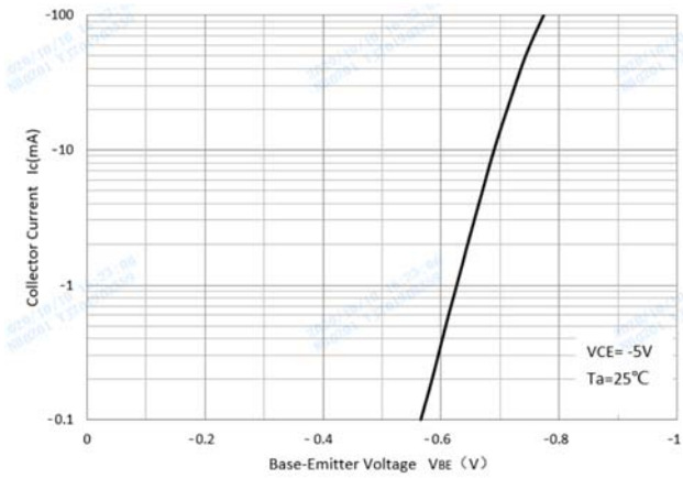
Fig 5: Base-emitter on voltage
